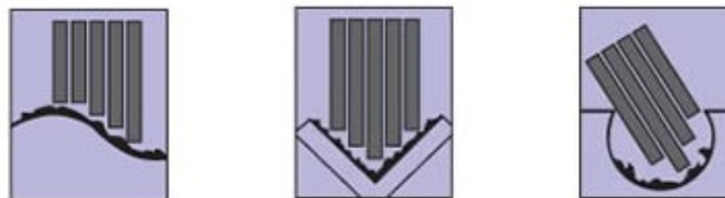
Figure 1.3 – Needles conforming to surface irregularities.
