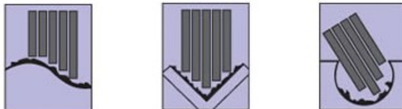
Figure 1.3 – Needles conforming to surface irregularities.
